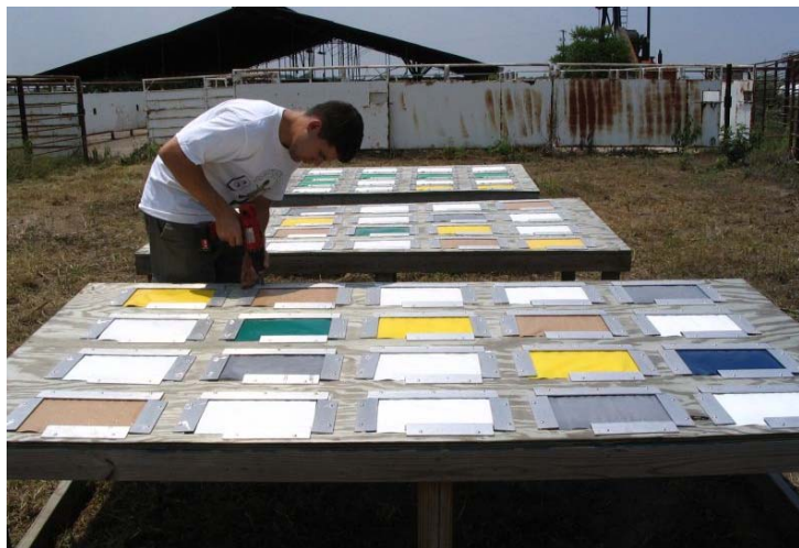
Figure 2: Outdoor weathering racks with module cover samples.
