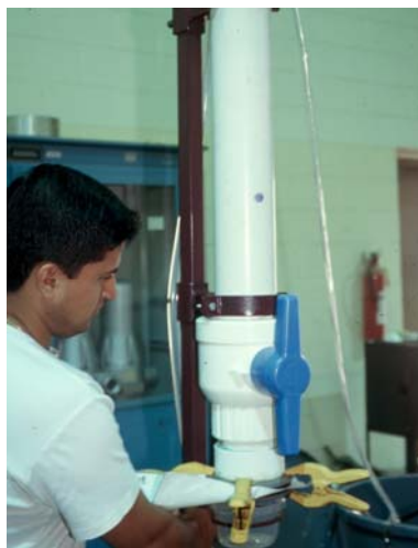
Figure 1: Ponding test apparatus.
